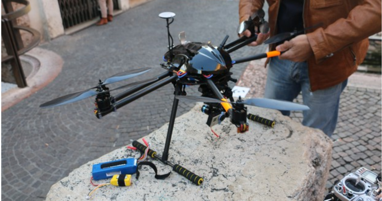
Figure 7. UAV and GoPro used to take aerial photos.
