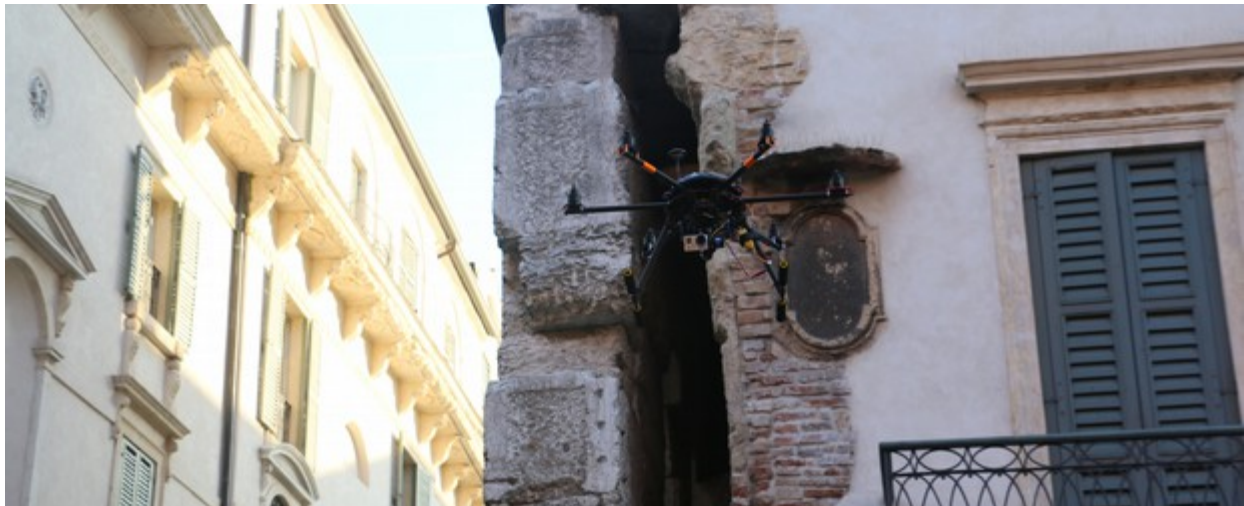
Figure 8. UAV and GoPro used to take aerial photos.
