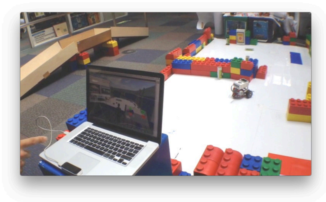
Figure 4. LEAP Motion controller being used for remote maneuvering of EV3 robot via OpenSim Training Area.
