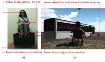
Figure 3. PhyMEL-WS. (a) Real image. (b) Virtual image in 3<sup>rd</sup> person mode
