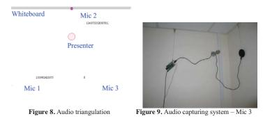
These microsystems are *Raspberry Pi®* devices driving a *Samson®* USB microphone chosen for its high gain and quality. The audio source location stream is transmitted by using *ffmpeg®* engine producing 3 different streams, one per microsystem. If more precise location algorithm is needed then a number of microsystems can be added to the overall system. The main audio, used during reproduction, is sent together with the RMTP video signal, through the Media Server.
