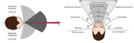
Figure 1. Horizontal Field of View.
