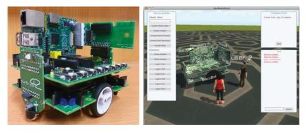
Figure 1. BuzzBoard Desktop Robot & screenshot of 3D Virtual interface.
